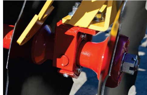
TRUNNION TYPE BEARINGS WITH STEEL PLATE FORGED BRACKETS
