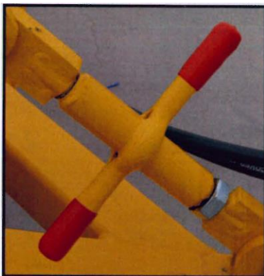
MOUNTED TURNBUCKLE ADJUSTS HITCH TO TRACTOR HEIGHT.
