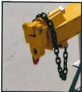
TONGUE SINGLE LIP IS STANDARD, DOUBLE LIP AND TONGUE PIVOT DROP OPTIONAL.
