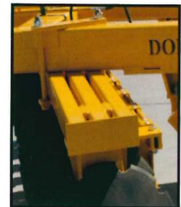
GANG BEAMS THREE 4" X 6" HEAVY WALL TUBE
