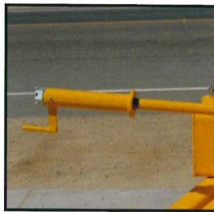
DEPTH CONTROL THREADED CRANK GIVES DEPTH OF CUT SETTINGS
