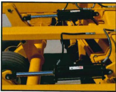
HYD. LIFT SYSTEM. DEPTH CONTROL RISE AND LEVELING UNIT
