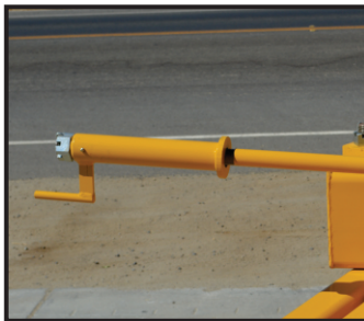
DEPTH CONTROL THREADED CRANK GIVES DEPTH OF CUT SETTINGS
