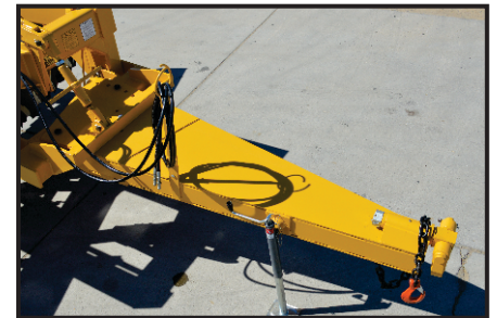
HITCH ALLOWS SHORTER TURNS BEHIND DUAL WHEEL AND TRACK TYPE TRACTORS
