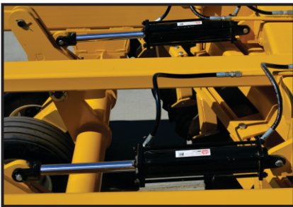
HYD. LIFT SYSTEM. DEPTH CONTROL RISE AND LEVELING UNIT
