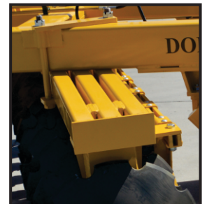
GANG BEAMS THREE 4" X 6" HEAVY WALL TUBE
