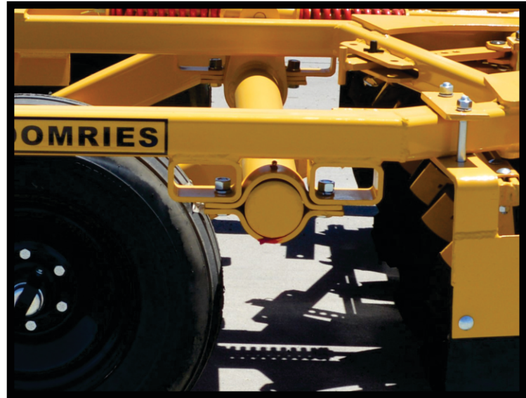
HEAVY DUTY AXEL SHAFT WITH 4 LUBRICATABLE BEARINGS.
