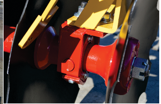
TRUNION TYPE BEARINGS WITH STEEL PLATE FORGED BRACKETS
