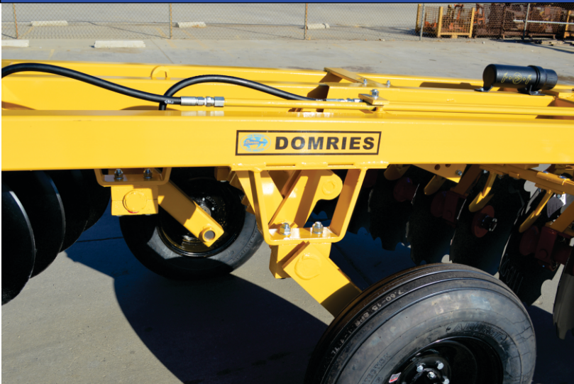
SPLIT AXLES ALLOW REGULATING THE DEPTH OF CUT FOR LEFT OR RIGHT SIDE
