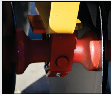
TRUNION BEARING WEAR PLATE AND HEAVY CAST IRON SPACER.
