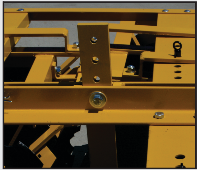
CENTER SHANK FOR CHISEL OR SWEEP
